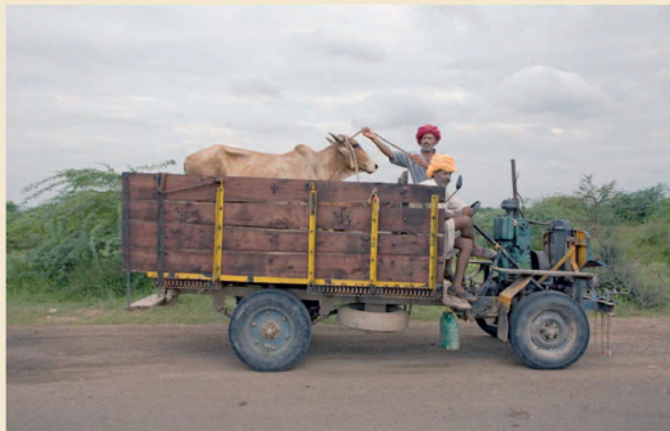
A jugaad vehicle—assembled entirely from spare parts, water pump engines, and wooden carts. The vehicle displays no registration plate, runs on diesel, and pays no road tax.
